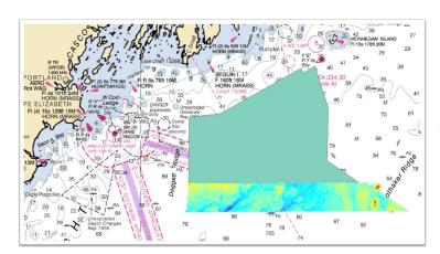
NOAA is conducting survey operations East of the Portland "Papa" buoy. The surveys will fill a long existing gap from the existing 1835 lead-line data which will be updated with a modern high resolution survey data. The survey will be facilitated by the NOAA ship Ferdinand R. Hassler sometime in 2020.
